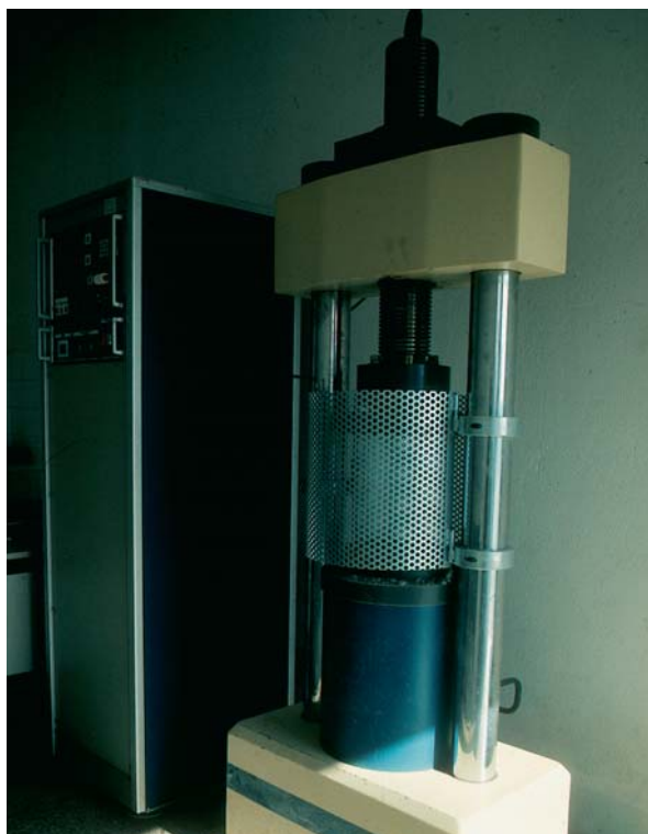
Trial for compression shear on concrete specimens
