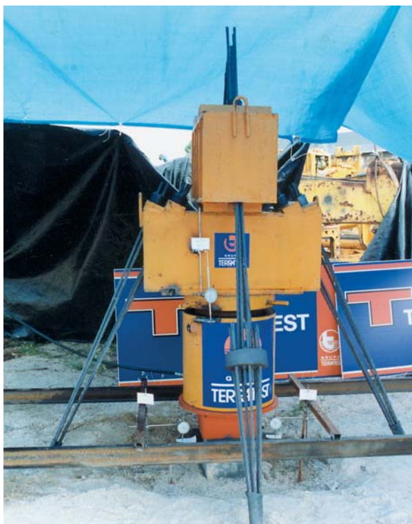
Static load test on a prestressed pile
